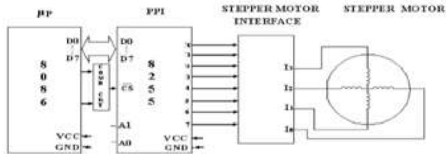
Fig: Interfacing stepper motor module to 8086 microprocessor
