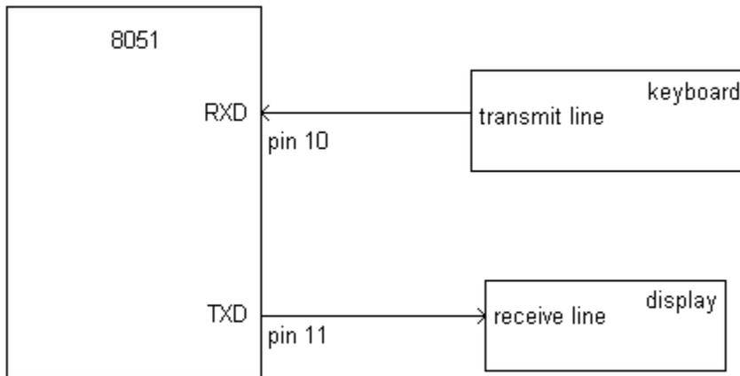
The TXD line is pin 11 of the microcontroller (P3.1) while the RXD line is on pin 10 (P3.0). Therefore, external access to the serial port is achieved by connecting to these pins. For example, if you wanted to connect a keyboard to the serial port you would connect the transmit line of the keyboard to pin 10 of the 8051. If you wanted to connect a display to the serial port you would connect the receive line of the display to pin 11 of the 8051. This is detailed in the diagram below.
